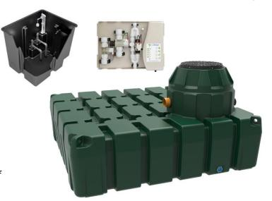
HydroStore "Home Harvest Gravity" rainwater harvesting systems connect a gravity fed plumbing system via a smart header tank to the pump within the tank, to provide recycled rainwater to the required water appliances such as toilets, washing machines and the garden.
